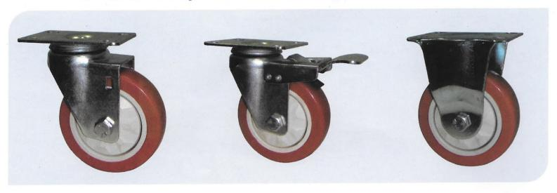
Polyurethane wheel - Made of Polyurethane wheel on precision ball bearing wheel center made of polyamide tread made of injected PU hardness 85shore A & 95 shore A Non- marking smoothness & Silence Plate Type Castor - Swivel castor with lock, housing made of pressed steel, bright zinc plated, double ball bearing swivel head, wheel axle with nut, dustguard.
