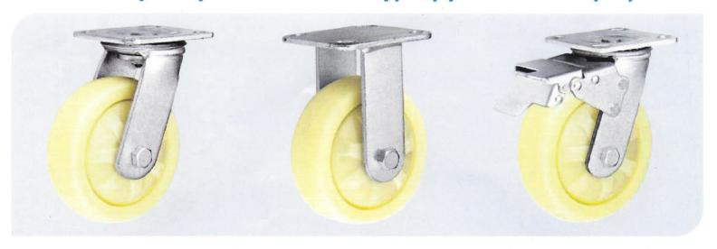
Polypropylene wheel - Centre made of Polypropylene, Tread: Polypropylene, White color wheel with Plain Bearing Plate Type Castor - Swivel castor with lock, housing made of mild steel, bright zinc plated, double ball bearing swivel head, wheel axle with nut, dustguard.
