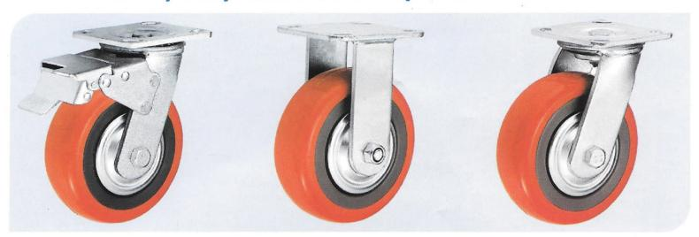
Polyurethane wheel - Made of Polyurethane wheel on precision ball bearing wheel center made of polyamide tread made of injected PU hardness 85shore A & 95 shore A Non- marking smoothness & Silence Plate Type Castor - Swivel castor with lock, housing made of mild steel, bright zinc plated, double ball bearing swivel head, wheel axle with nut, dustguard.
